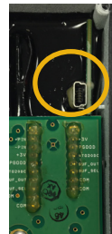
Figure 1. The USB connector is found on the bottom of the MX2034. Remove the back plane of the MX2034 to access it.
