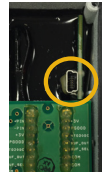
Figure 1. The USB connector is found on the bottom of the MX2034. Remove the back plane of the MX2034 to access it.
