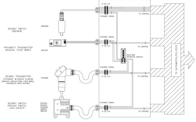
NOTE: SEE THE WIRE SIGNALS OF EACH PRODUCT FOR CONNECTION TO MONITORING AND CONTROL DEVICES.
