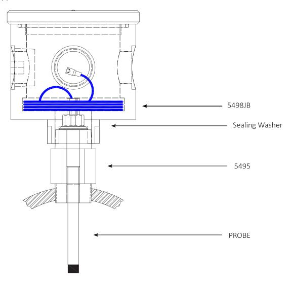
The  $\frac{3}{4}$ " NPT thread on one side of 5495 Forward Mount Probe Holder is used to connect 5498JB, and the other side with either  $\frac{3}{4}$ " or  $\frac{1}{4}$ " NPT thread is used to mount on machine case.
