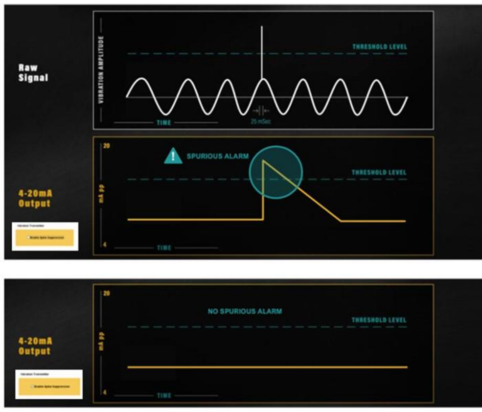
FIGURE 15 – Example of how Spike Suppression prevents an electrical spike from impacting the 4-20 mA signal.
